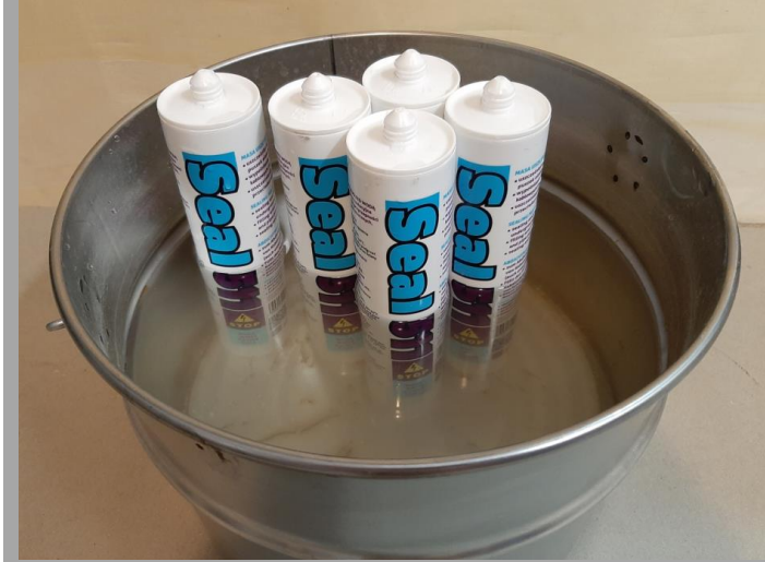
STEP 1: PRIOR TO APPLICATION, PREHEAT THE CARTRIDGES UP TO 30÷40°C.
