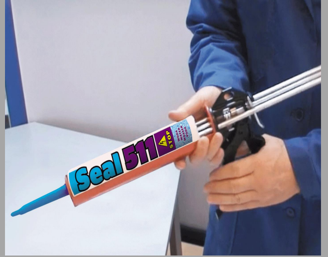
STEP 2: INSERT THE PRE-HEATED CARTRIDGE INTO THE INJECTION TOOL AND INSTALL APPROPRIATE NOZZLE.
